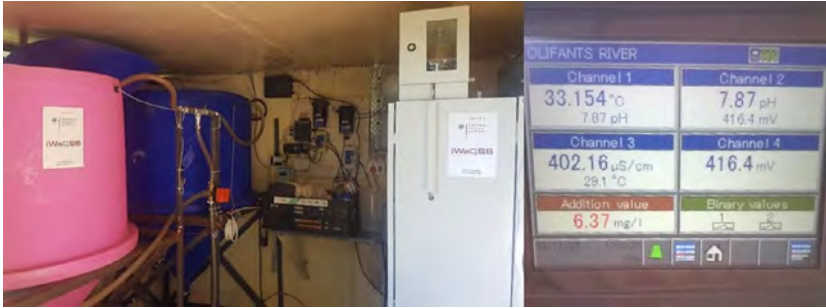
Fig. 11 Real-time water quality monitoring including sediment samplers and sensors for toxicity monitoring, pH, Conductivity and additional parameters.
